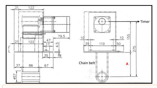
Customers provide the dimension A in order to decide the steel belt length for manufacture.
