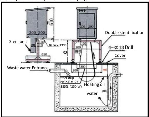
Customers provide the dimension A in order to decide the steel belt length for manufacture.
