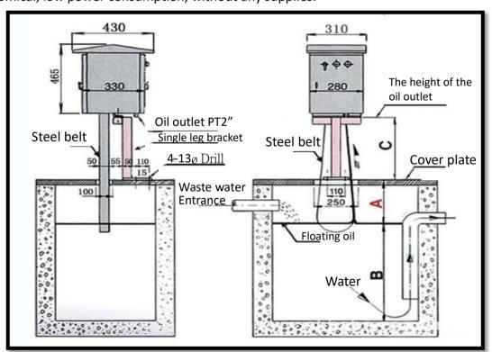
Customers provide the dimension A in order to decide the steel belt length for manufacture.
